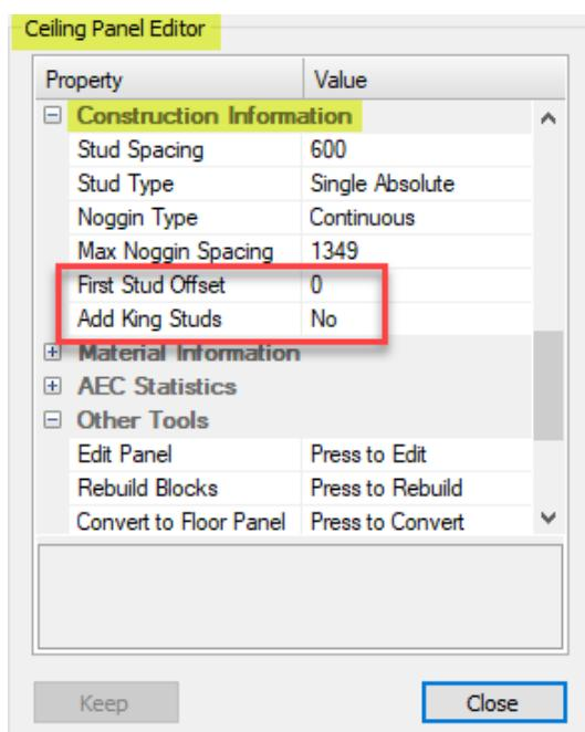
8. If the 'Stud Type' is set to use absolute spacing, then the 'First Stud Offset' can be applied. The offset distance is taken from the left-hand end of the panel to the centre of the first stud. If the 'Stud Type' is set to use even spacing, then the first stud offset will not be applied.
