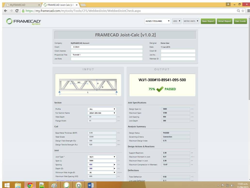
Otherwise, after step 10, you can draw a joist in Steelwise using the ADD command and alter the parameters to suit the worst-case scenario to establish your joist materials, spacing and depth.
