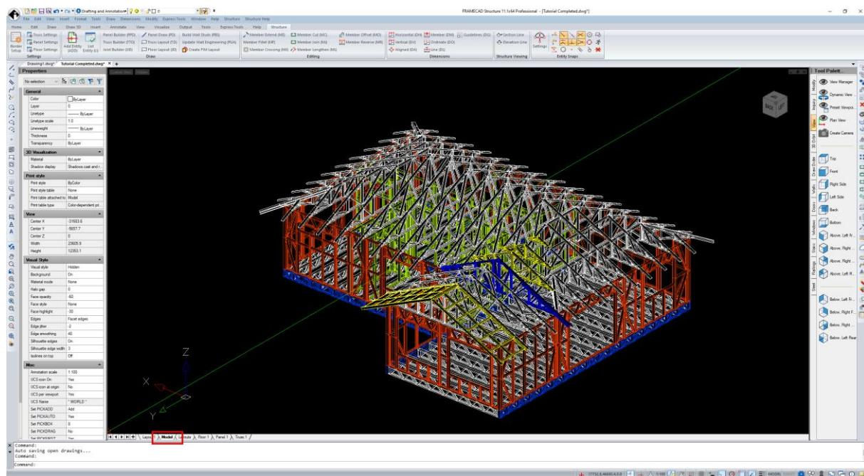
**Detail Space:** Used to display detail drawing sheets of each generated frame.
