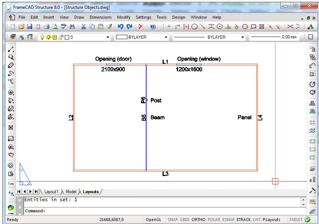
Panel Layouts can also include two Member Objects which are part of the detailed Wall Panel Frames (refer to Detailing Space Objects)
