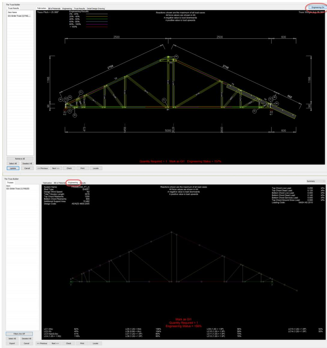
7. Some parameters can be modified by double clicking on the truss name in the left column of the Truss Builder. Make changes, Amend, and then Update.
