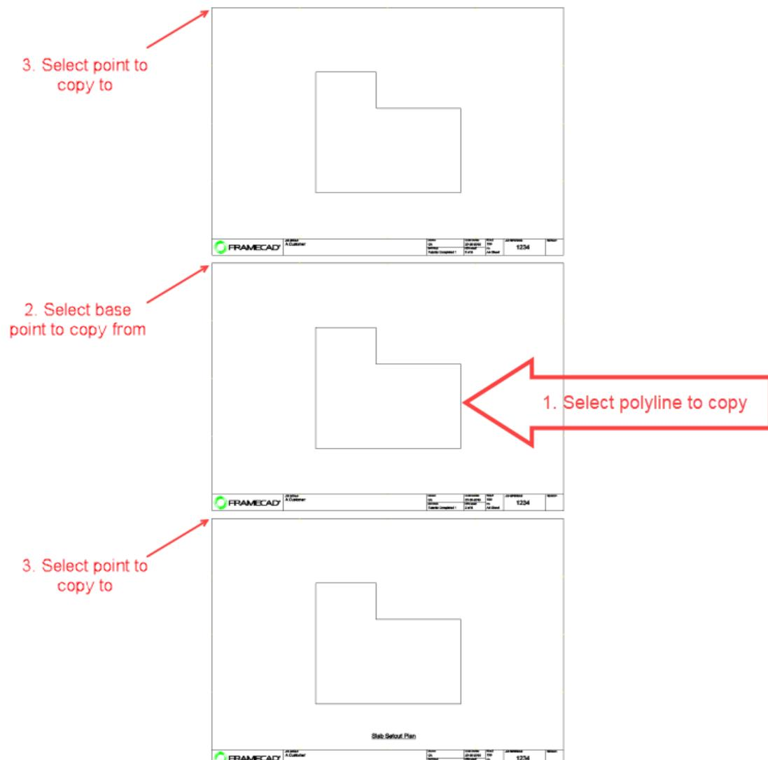
**11. NOTE: It is recommended that the outline is copied to the exact same location within each border by selecting a base point to copy from and selecting the same locations on the other borders to copy to. Use a corner of each border as the 'base point' and the 'copy to' point.**
