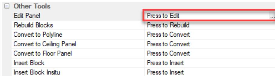
5. Blocks can also be displayed in the layout plan by clicking on the 'Insert Block Insitu - Press to Edit' button in 'Other Tools'.
