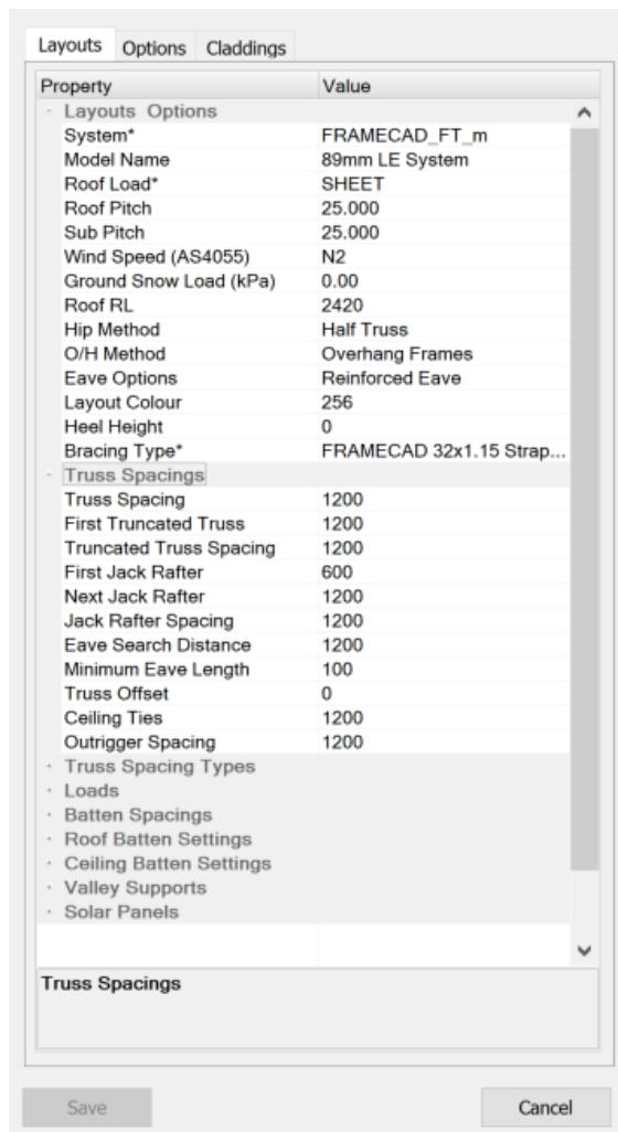
g) After changes have been made to the settings, they will be maintained for future jobs unless you change either the System, Model or Roof Load. However, you can permanently save these for future use by holding down the 'ALT' key and clicking on 'System\*'. These settings will be saved to a user defined data file which can be updated at any stage by repeating the above procedure.
