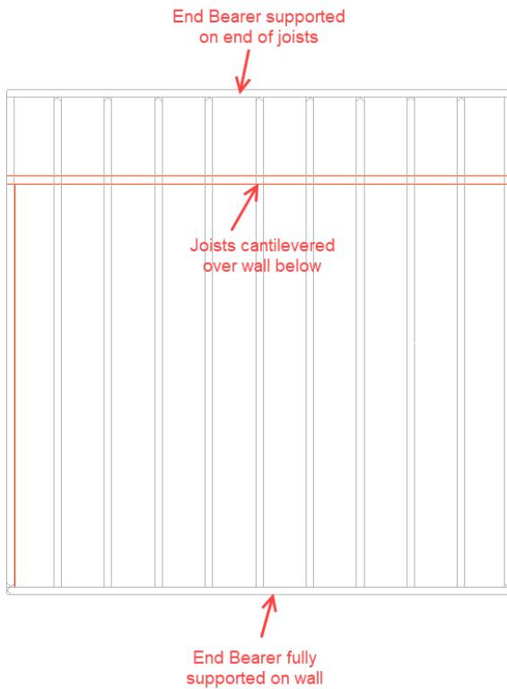
In the example above, the member on the cantilevered end of the joists will remain as an End Bearer because it is supported by the joists.
