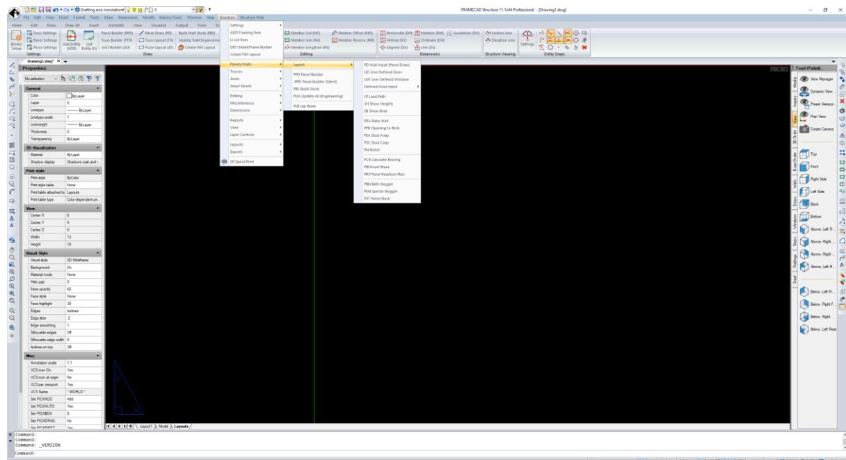
A **Ribbon Bar** appears below the menu bar. These are effectively customised toolbars that provide easy access to common commands. Users should select the "Steelwise" Ribbon for general use.
