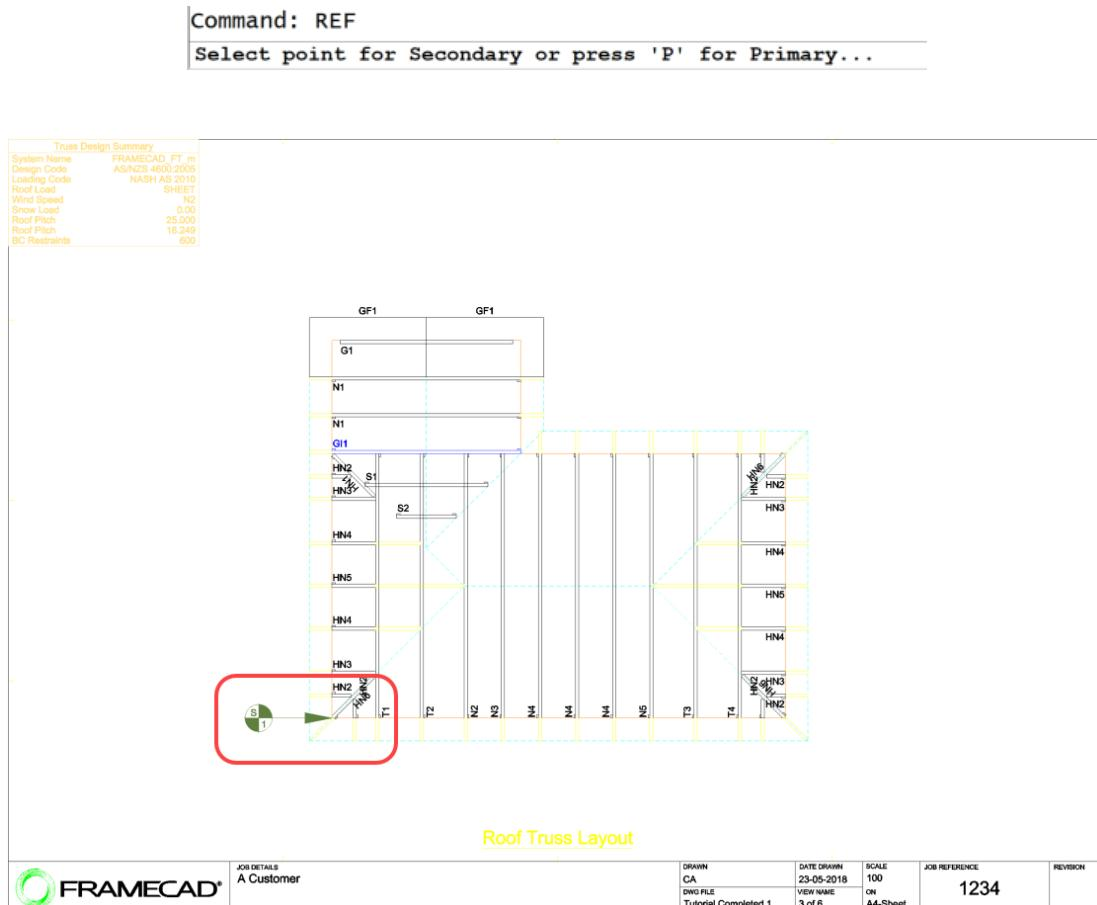
**Remember – no part of a reference marker must be outside of a border.**
