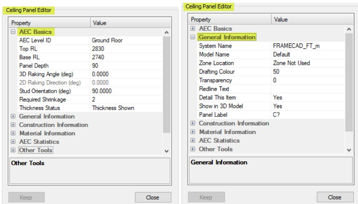
9. 3D Raking Angle determines the sloping pitch of the panel.
