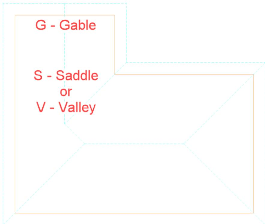
9. Create the Truss Layout using Truss Draw (**TD**) by selecting Roof Blocks on the Support Lines (Orange Lines only) using the same input method as per the Roof Line input. Select the same roof type options as you did for the Roof Line input.
