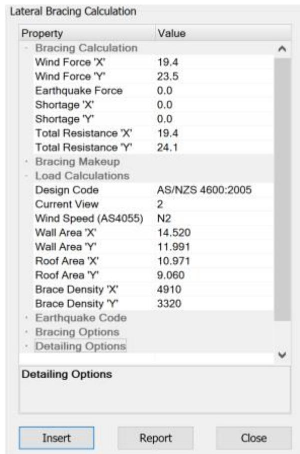
8. To create a Bracing and Racking Resistance Plan, ensure that the Wall Layout Plan is in focus on the screen, then re-activate Panel Calculate Brace (**PCB**). In the PCB form, go to Detailing Options and select 'Create Bracing Plan' then click on 'Insert'. The plan will zoom to extents to display all the borders, then select an empty border to create the bracing plan in.
