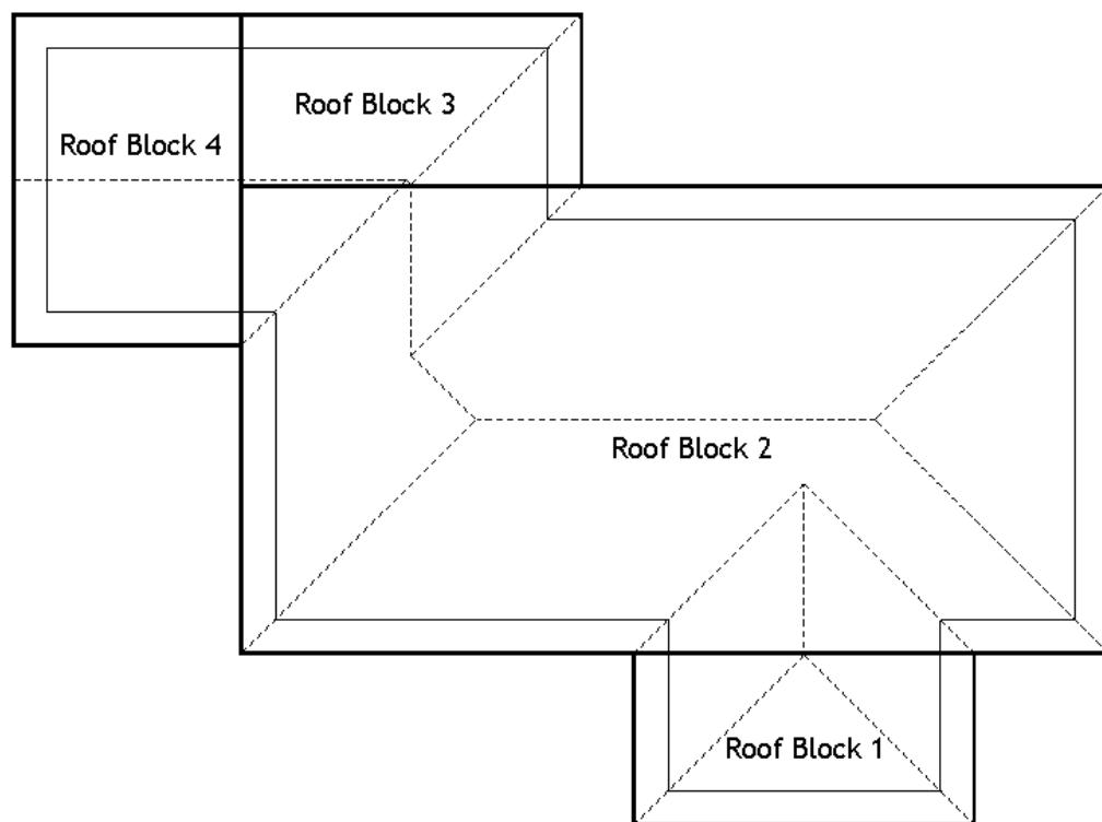
The example below shows a good example of a complex roof. Note the overlap of the two roof blocks. Generally, when you have an overlap of roof blocks, you have a complex roof. The larger the overlap, the more complex the roof.
