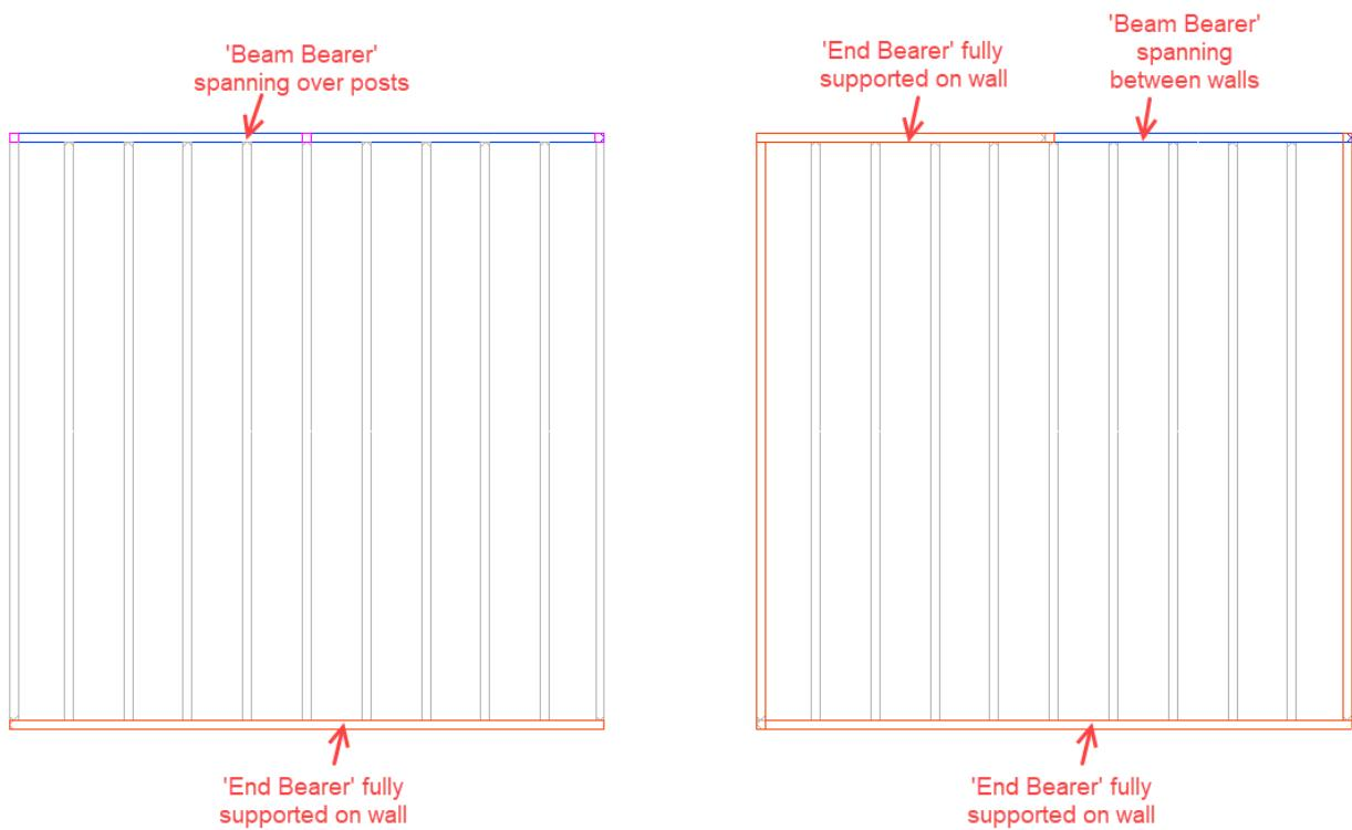
In the second example above, the End Bearer has been split into two members, so the unsupported portion can be defined as a Beam Bearer.
