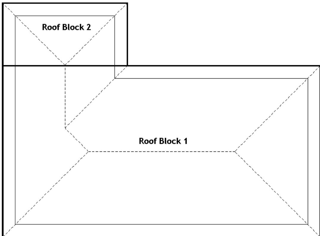
Where the entire roof is of one pitch, all roof lines will be at right angle to each other, with the hips and valleys at 45° angles.
