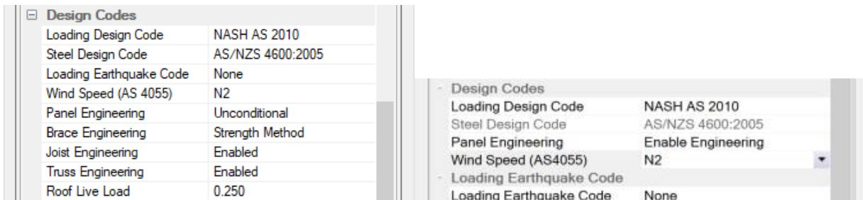
The screenshot shows the 'Design Codes' configuration in the software. The left panel displays the current settings, and the right panel shows the configuration after changes have been made. The changes include setting 'Steel Design Code' to 'AS/NZS 4600:2005', 'Panel Engineering' to 'Enable Engineering', and 'Roof Live Load' to 'None'.
