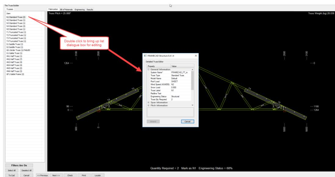
3. Click on 'Select All' and then 'To CAD' to export trusses. A new Detailing space tab is created labelled 'Truss.1'.
