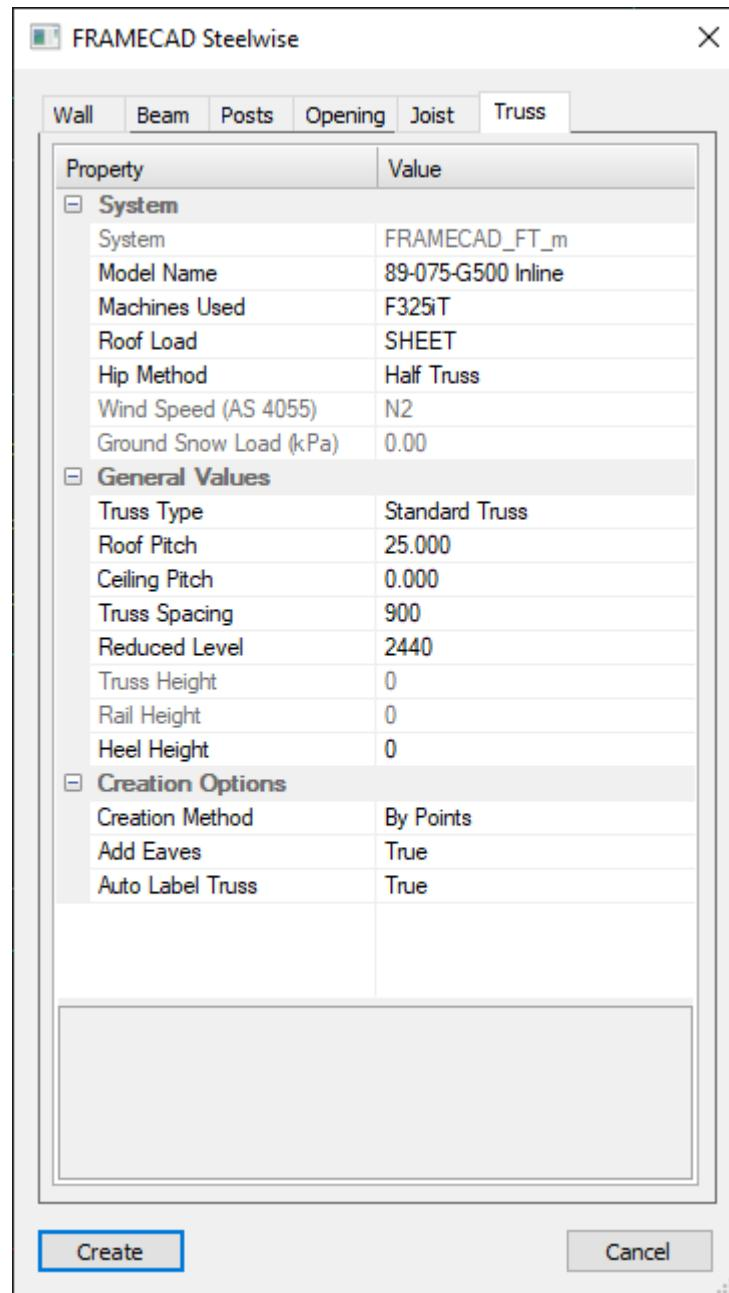
13. To edit a truss after it has been placed, use List (**LI**) to bring up the truss properties.
