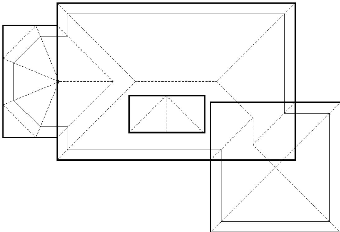
Note the direction of fall. On each occasion the roof MUST fall to a valley or gutter.
