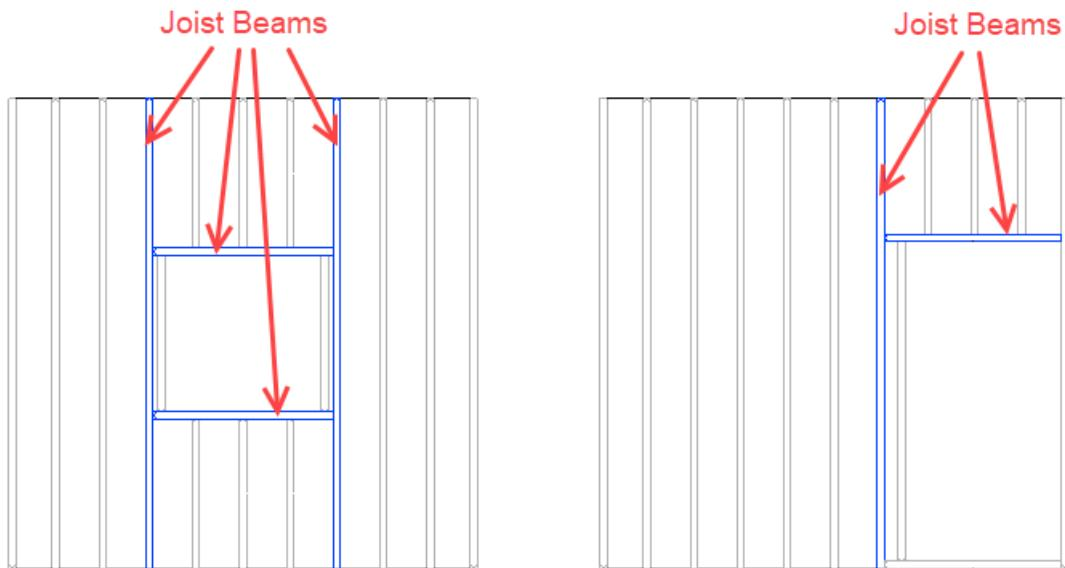
**Beam Bearer** – this is defined as an End Bearer that supports Joists and Joist Beams, but spans between two or more supports, whereas an End Bearer is continuously supported. See examples below.
