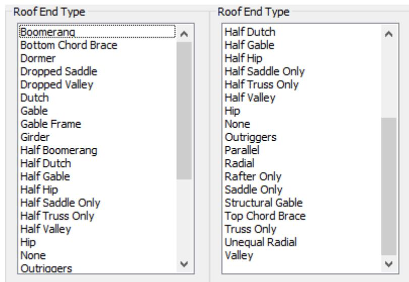
E.g. if the user wishes to create a mono pitch roof using half trusses, type **M** for more options and double click on 'Half Gable' or type **HG** at the Roof Type selection.
