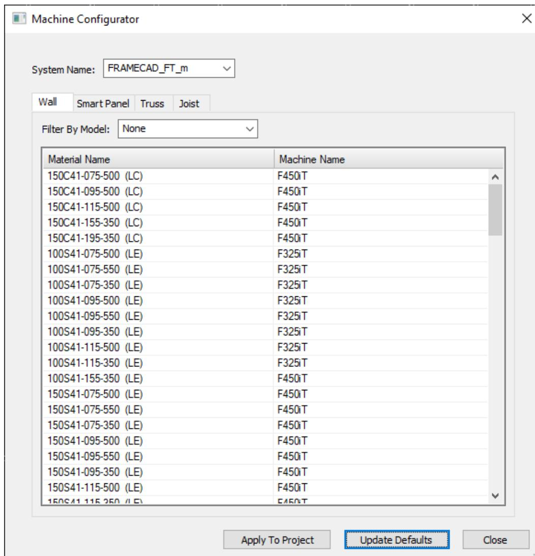
The Machine Configurator shows the System Name and all the material that is able to be rolled and the associated available machines. This allows you to modify which machine is used to run each profile. You will need to do this for each frame type: Wall, Smart Panel, Truss, Joist. The available profiles can also be filtered down by the framing Model.
