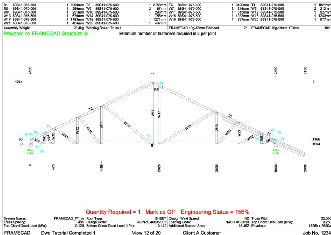
6. To see where the member is failing, click on the 'Engineering Off' button on the top right corner of the Truss Builder. This will then change to 'Engineering On' and coloured lines indicating engineering results will be superimposed over the truss. Any red lines indicate where the member failures occur.
