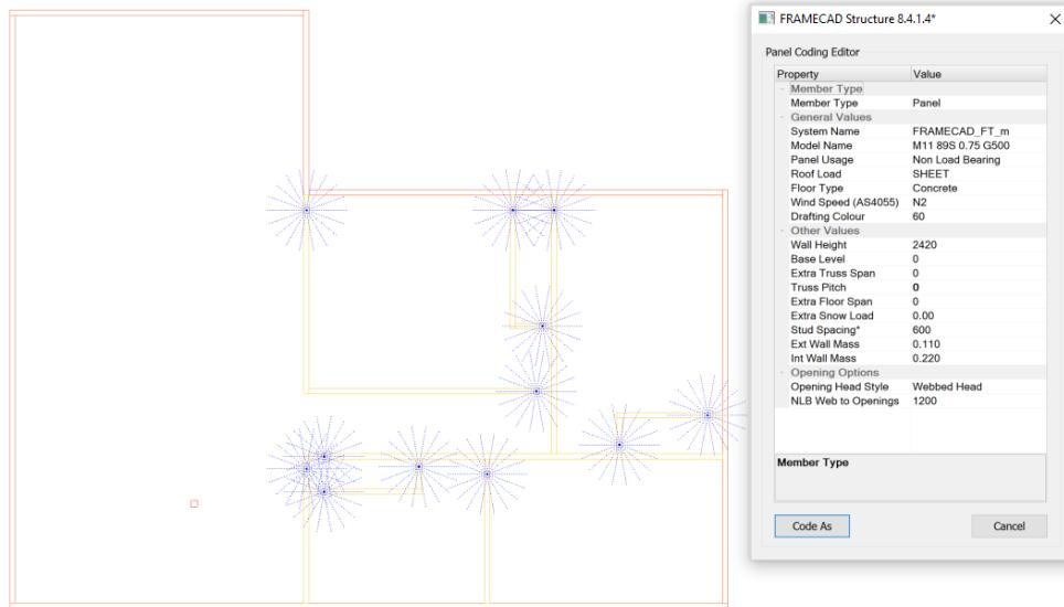
10. When listing non-coded panels - define the initial values such as member type (Panel or Beam), panel usage (Load Bearing, Structural Only or Non-Load Bearing), wind load, frame height, base level and other settings. Click on 'Code As'.
