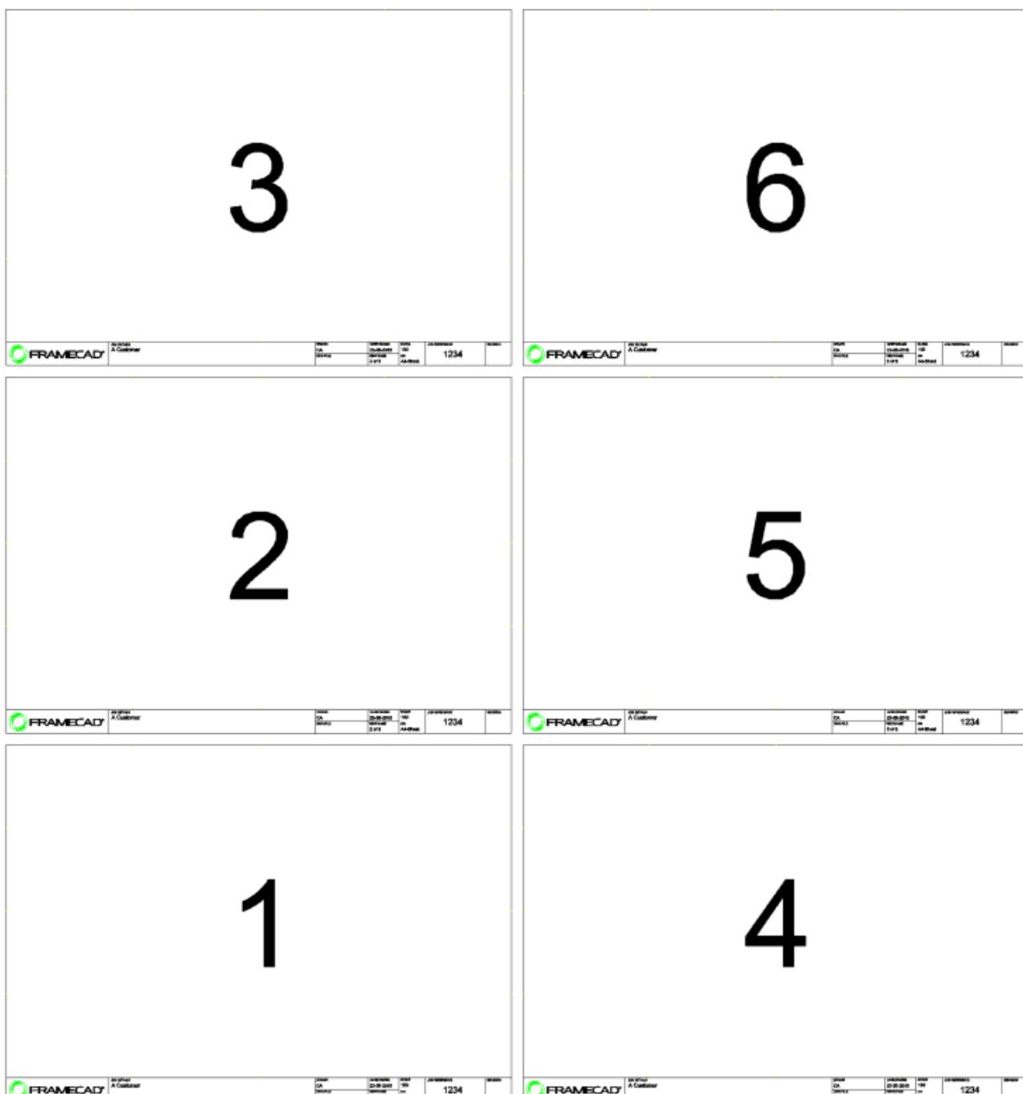
**Once the layout borders have been inserted, the location or size of the borders must not be changed.** It is, however, possible to add or remove layout borders to the selected space by running the BSET command again and editing the 'Quantity'.
