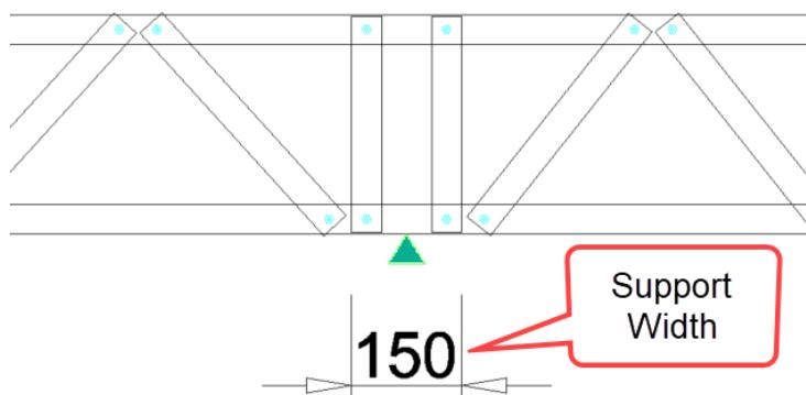
To apply a width to a support line, list (LI) the support line and change the ‘Support Line Data’ parameters to suit (see below).
