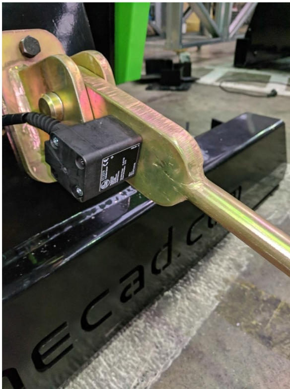
Figure 1. Inclinometer installed on dancer arm pivot.
