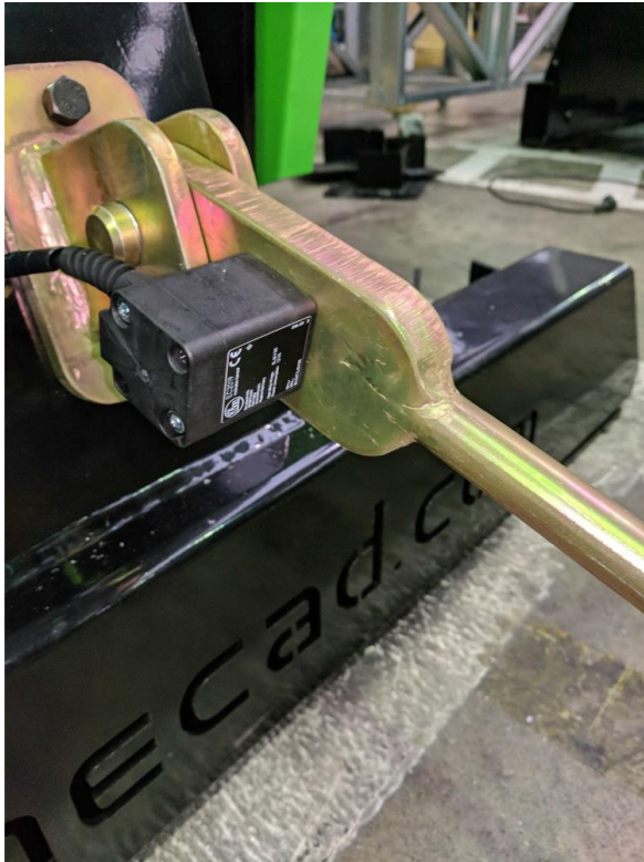
Figure 1. Inclinometer installed on dancer arm
