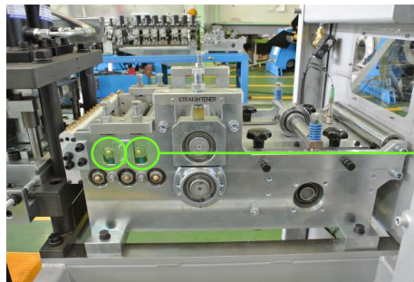
Top Rollers: Reverse steel strip out until clear of the top rollers
