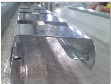
An Example of Incorrect Flange Height
