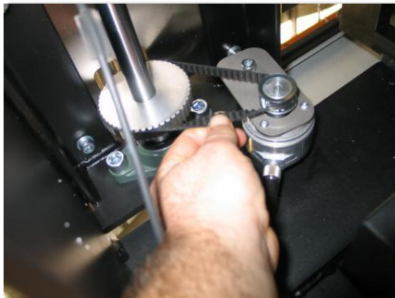
Encoder Belt Tension Test
