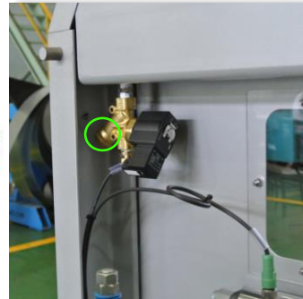
The two types of filtering used on the TF550H lubricant: left – in-line filter, right – filter in base of lubricant delivery solenoid
