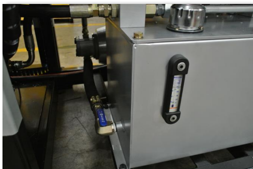
Hydraulic tank with level indication
